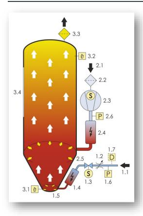
Ambient air (2.1) is drawn in by a speed-controlled blower (2.3) through an air filter (2.2), heated up in the heater (2.4) and blown into the drying hopper through the distributer ring for ambient air (2.5). Pre-dried compressed air (1.1) is supplied by a quick connector. It
