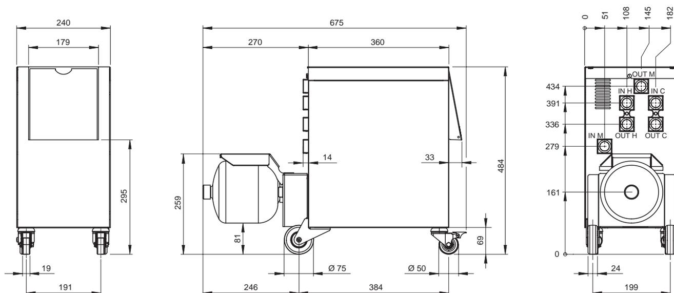
IN H Input hot water circuit
